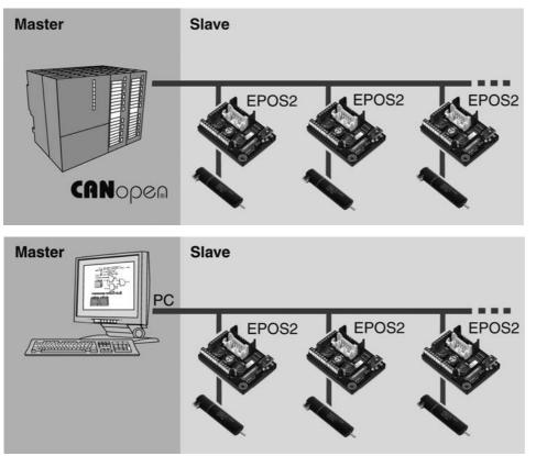
EPOS2 is a modular constructed digital positioning controller. It is suitable for DC and EC motors with incremental encoder with a power range from 1 to 700 watts.
